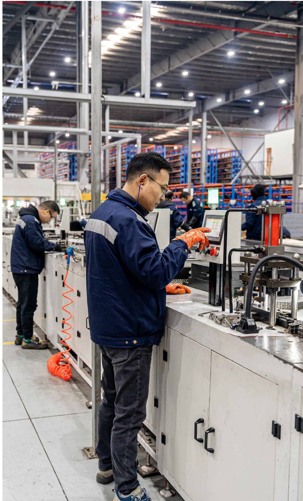
Set-up technician checks chain cutting parameters at our facility in Jintan, China
