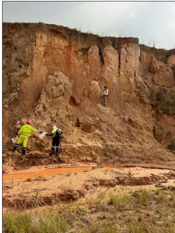
Figure 12 and 13. Thick clay dominated, deeply weathered regolith over parts of the main Benga Novo intrusion.
