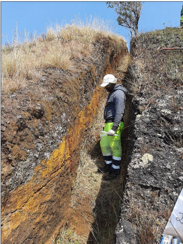
Figure 7 and 8. Channel sampling laterite exposed in Trench 1 (68 m) and Pit 1 (6 m) at Sulima West.
