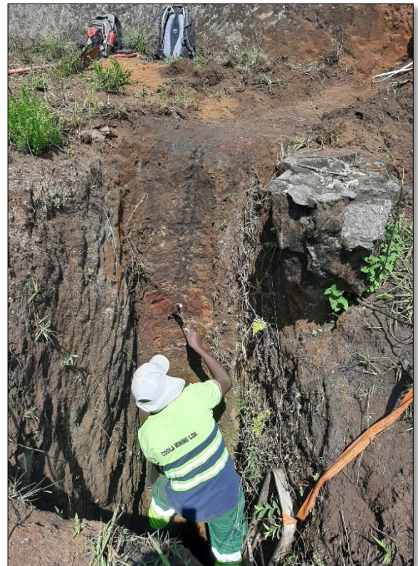
Figure 7 and 8. Channel sampling laterite exposed in Trench 1 (68 m) and Pit 1 (6 m) at Sulima West.
