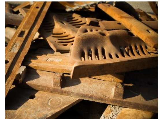
Mill steel liners
