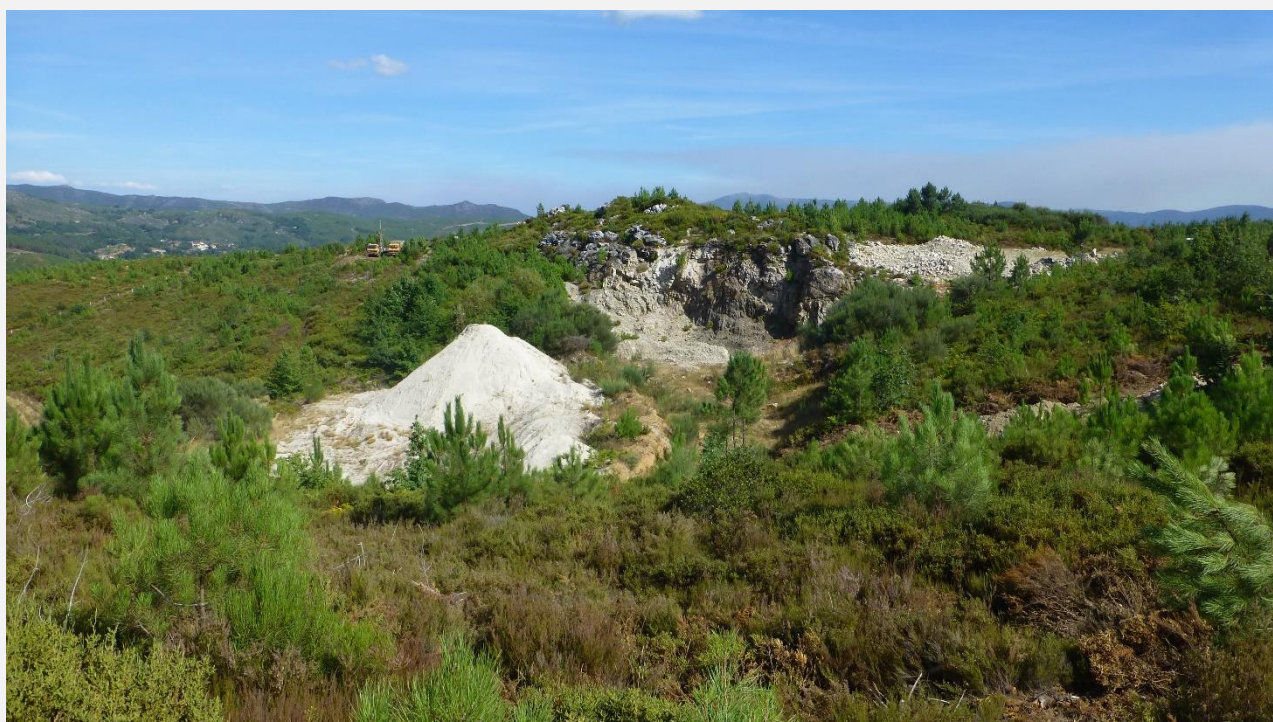
Figure 6. Small bulk sample pit on lithium bearing pegmatite on the NOA prospect
